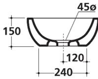
The M2 above counter basin is the quintessential vessel type basin. Substantial but elegant, beautiful but functional and perfectly proportioned to suit many applications. The 350mm front to back dimension allows you to use either wall mounted or bench mounted tower style tapware.
