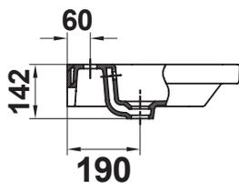
The Street Square 60 wall-hung basin with overflow, made by Gala of Spain, captures the essence of fine European sanitaryware. This basin can be installed over counter or wall-mounted.
