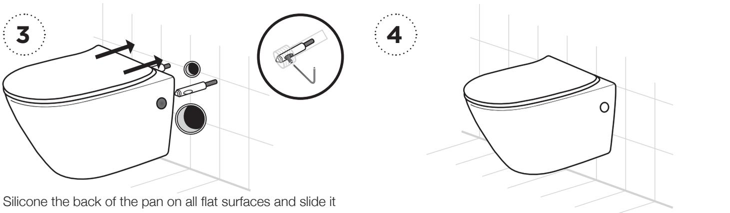
Silicone the back of the pan on all flat surfaces and slide it onto the brackets, so it is pressed right up against the wall. Using an allen key, tighten the grub screws on both sides of the pan to lock it in place.
