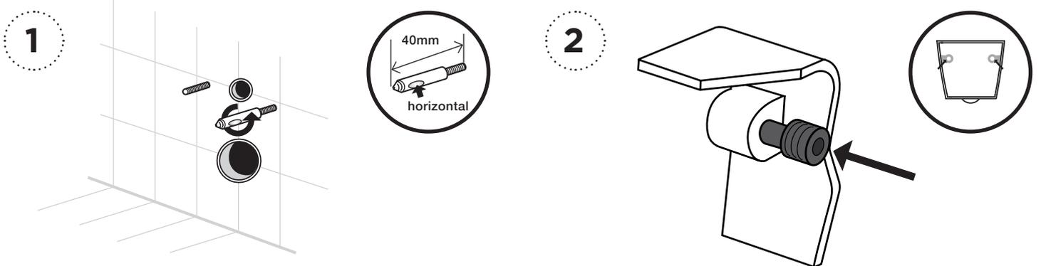
Screw the threaded sockets onto the metal supports of the cistern frame until the entire length of the metal support **plus** the threaded sockets measures 40mm. Make sure the hollow indentation is facing outwards.
