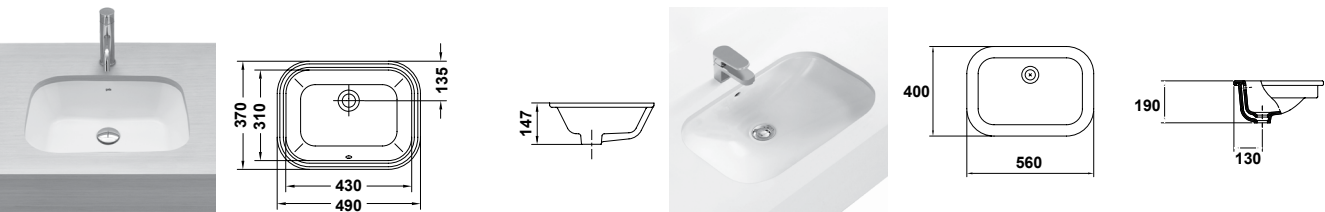
26020 Flex under counter 49 x 37cm basin Features integral overflow Supplied with pop-up waste Capacity: 4.5L
