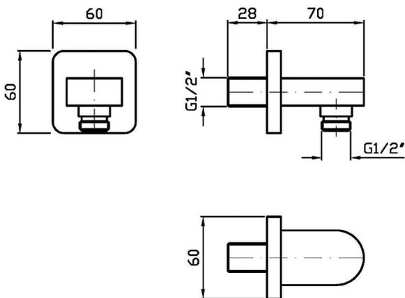
Wall elbow with 1/2" male water inlet connection. Crafted from solid brass.
