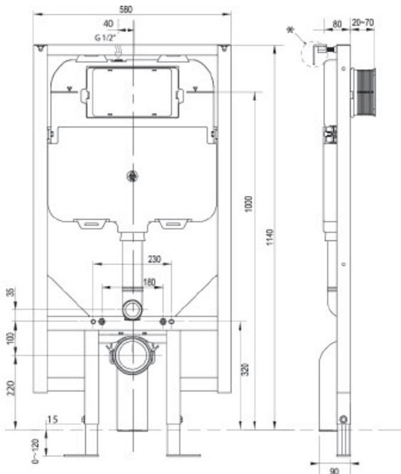
The concealed, dual flush cistern with frame is made from high density polyethylene, incorporating inbuilt overflow. This cistern is suitable for in-wall and under counter installation.
