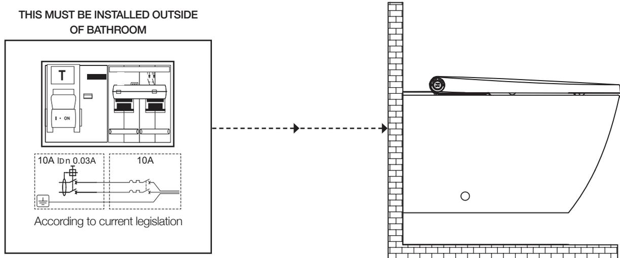
NOTE: Any electrical work conducted on this product must be installed by a qualified person in accordance with AS/NZ 3000 Wiring Rules.
