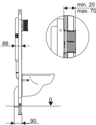
**Important:** the front face of the pan bracket must be flush with the front face of the studs. Bracket is suitable for use on non compressible wall materials only. Installer must ensure that the frame is fixed appropriately to structure to be able to support 400kg on the pan.
