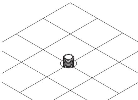
**4. Push on spout. Mark 4 holes on floor. Unscrew flange, align holes. Drill Ø6mm holes, screw flange back onto spout.**
